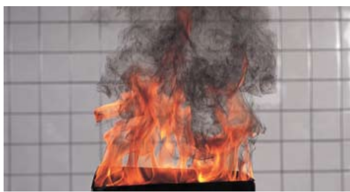
Test fire 5: liquid fire (n-heptane)
