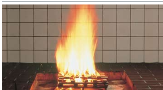
Test fire 1: cellulose open fire (wood)
