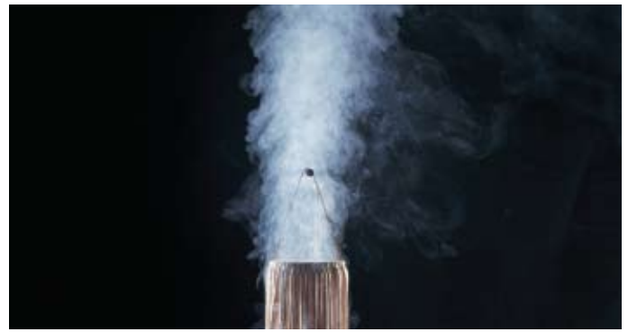
Test fire 3: glowing smoldering fire (cotton)
